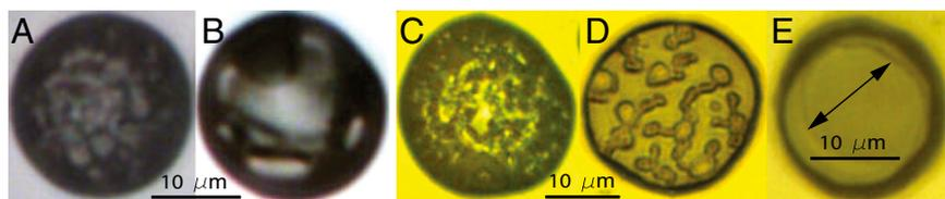
**Fig. 1.** Optical microscope images of (A and B) 20 wt%  $H_2SO_4$  drop at 183 and 214 K, respectively, (C) 25 wt%  $(NH_4)HSO_4$  at 243 K, (D) 35 wt%  $(NH_4)_3H(SO_4)_2$  at 257 K, and (E) 20 wt% citric acid at 218 K. The arrows show the border of ice core.
