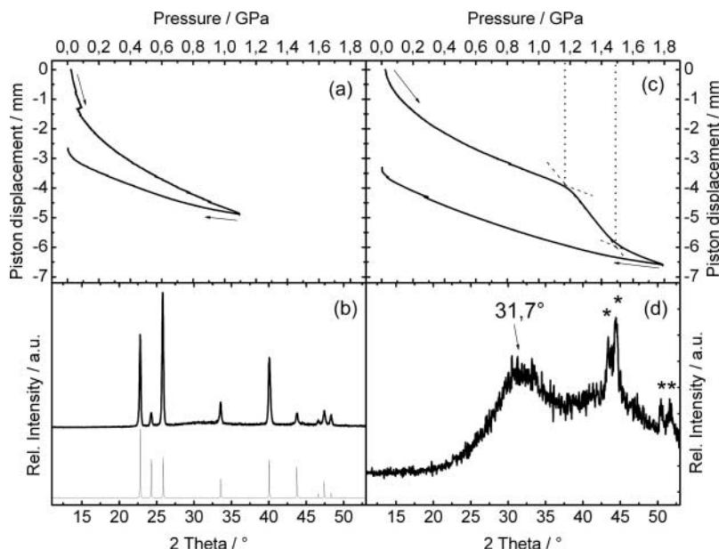
Figure 1. (a) Piston displacement and (b) black line (top): XRD ( $\text{Cu K}\alpha_1$ ) of sample 1 (quench-recovered from 1.1 GPa); blue line (bottom): calculated XRD of hexagonal ice; data from [4]. (c) Piston displacement (with  $p_{\text{onset}}$  and  $p_{\text{end}}$  of PIA marked by dotted lines) and (d) subsequent XRD of sample 2 (quench-recovered from 1.8 GPa). The asterisks mark the reflexes of the XRD sample holder.
