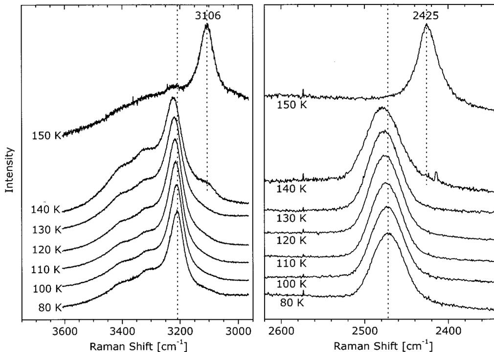
**Figure 3.** The temperature dependence of the peak frequency of the decoupled O–D stretching transition of H<sub>2</sub>O ice XII containing 9.0 mol % HOD, and the transition to cubic ice. The spectra are shown on the same ordinate scale, but are shifted vertically for clarity.
