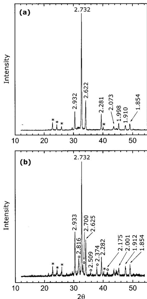
**Figure 1.** (a) X-ray diffractogram (Cu-K $\alpha$ ) of a pure ice XII sample with  $d$  spacings in Å, and (b) of an ice XII sample containing a small amount of ice IV (marked by open circles). The samples were recovered after decompression under liquid N<sub>2</sub> and diffractograms recorded at 80 K. Bragg peaks of ice Ih from condensation of water vapor during the transfer of the sample are marked with asterisks.
