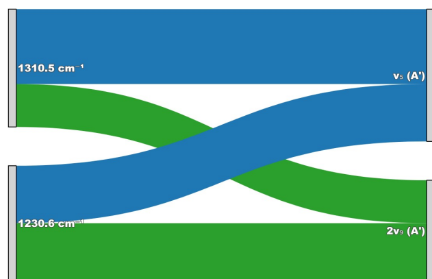
Fig. 2 Calculated resonance pair between the fundamental \nu_5 ( A' ) (blue) and the overtone 2\nu_5 ( A' ) (green) for HCOOH from the VCI calculation. The line width indicates the contribution of a given state to the VCI solution.
