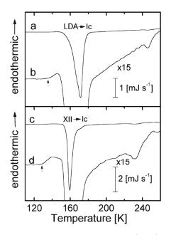
Fig. 13. – Glass transition of low-density amorphous ice (LDA) superimposed by the crystallization to cubic ice (depicted on the top). Endothermic step (transformation) in ice XII superimposed by the crystallization to cubic ice (shown on the bottom). Reproduced from ref. [74].
