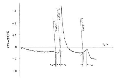
Fig. 14. – Differential thermal analysis curves for vapor deposited amorphous solid water. Reproduced from ref. [180].
