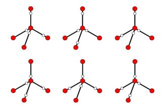
Fig. 3. – Six possible molecular orientations of a central water molecule in the Walrafen-pentamer, *i.e.*, a central oxygen atom (red) tetrahedrally surrounded by four oxygen atoms (red). These six configurations, but no others, can be obtained by distributing four protons (white) in accordance with the Bernal-Fowler rules. Each proton may sit on one of two possible positions along the line connecting two oxygen atoms (black lines), and there must be one proton sitting on each line.
