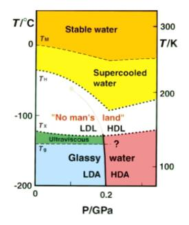
Fig. 11. – Phase diagram of metastable amorphous ices and liquid water. The solid black line depicts the phase boundary between LDA and HDA. Reproduced from ref. [176].
