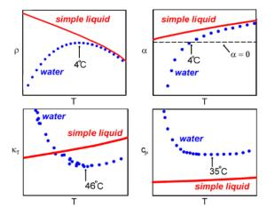
Fig. 7. – Isobaric temperature dependence of the density, the thermal expansion coefficient, the isothermal compressibility and the isobaric heat capacity for water (blue dotted line) and for a simple liquid (red line). Reproduced from ref. [146].
