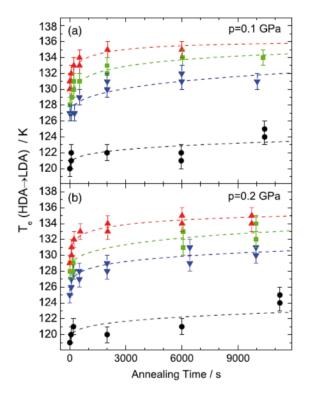
Fig. 19. – Calorimetric HDA-to-LDA transition temperatures  $T_e$  as a function of annealing time and temperature (110 K black circles, 125 K blue downward triangles, 130 K green squares, 135 K red upward triangles). The dashed lines depict the relaxation-function fits. Reproduced from ref. [201].
